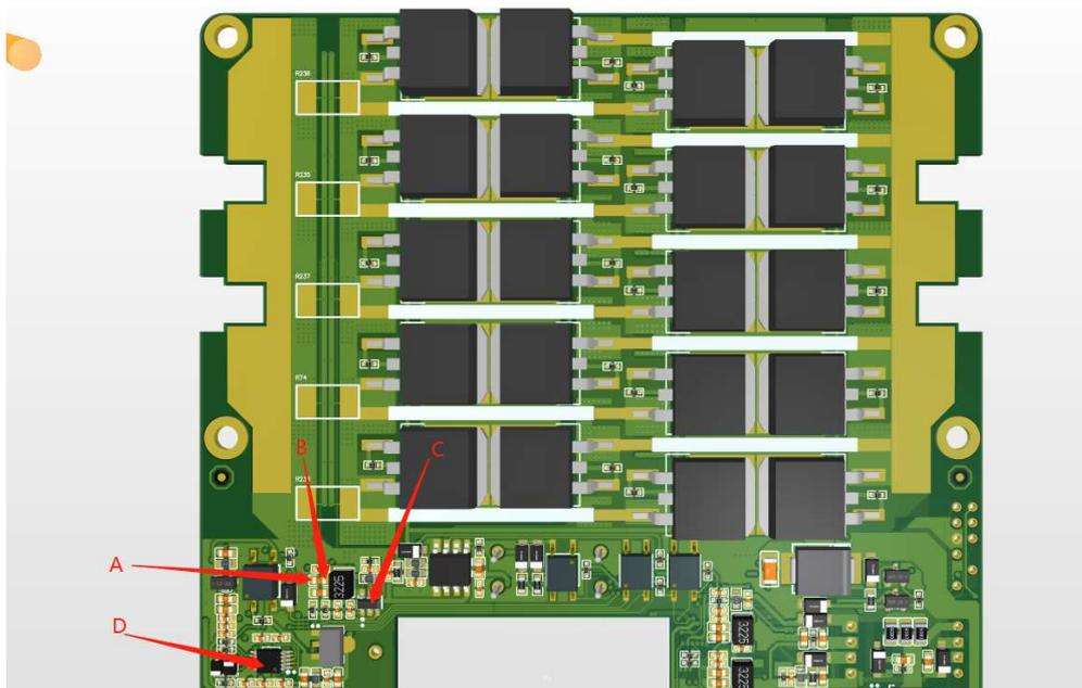
**Step 2:**After power on, test the voltage between A and B points in the diagram. If the voltage is between 4.5~5.2V, it is necessary to replace chip D, which is MDT10F272. After switching off and replacing the chip, turn on the machine again to test whether the functional fault is eliminated.
