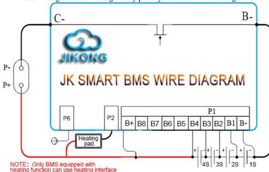
figure.8. wiring mode of 4-string battery pack system
