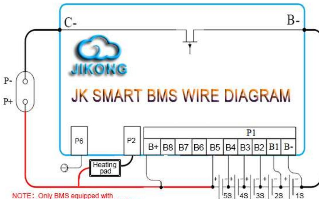
figure.6. wiring mode of 5-string battery pack system
