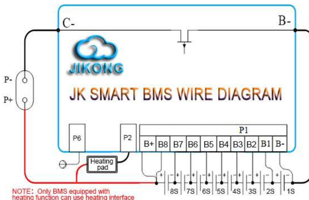
Figure 4. wiring mode of 8-string battery pack system
