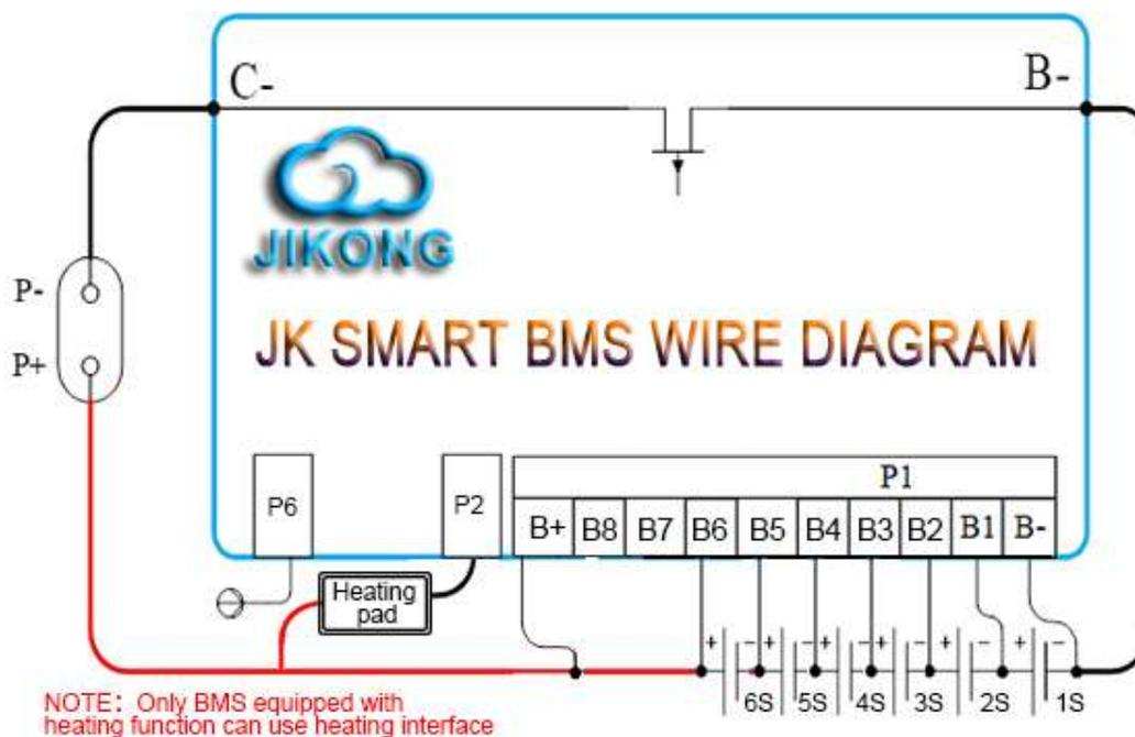
figure.6. wiring mode of 6-string battery pack system
