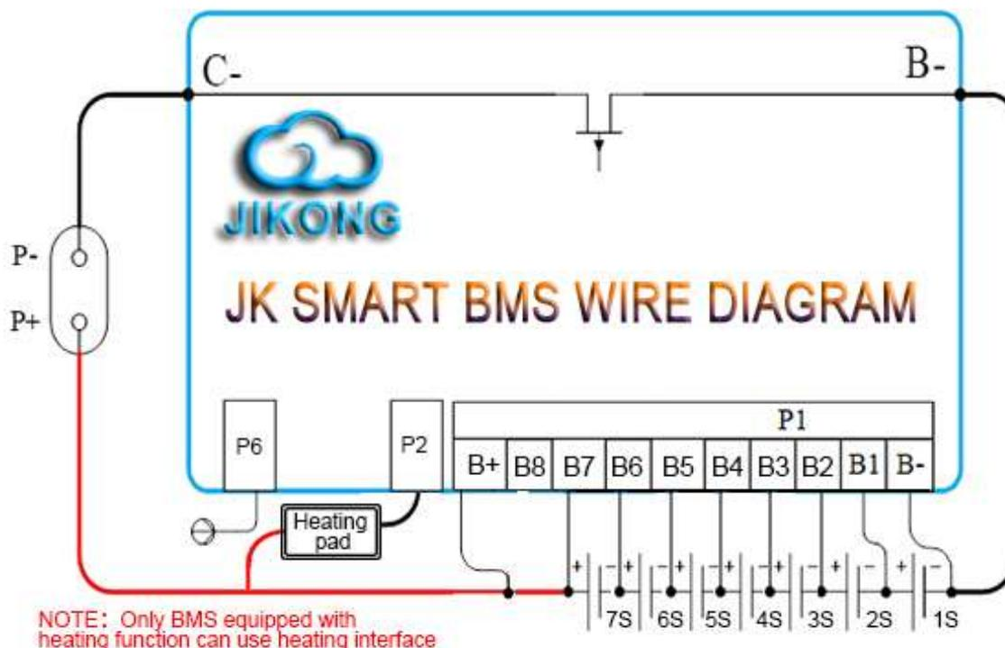
figure.5. wiring mode of 7-string battery pack system
